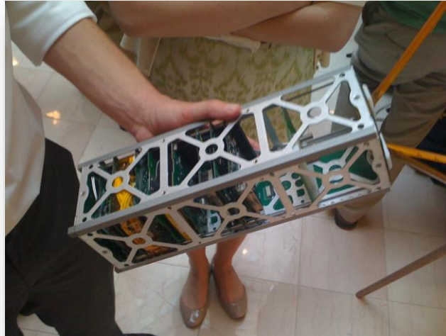
Standard 3U cubesat chassis
